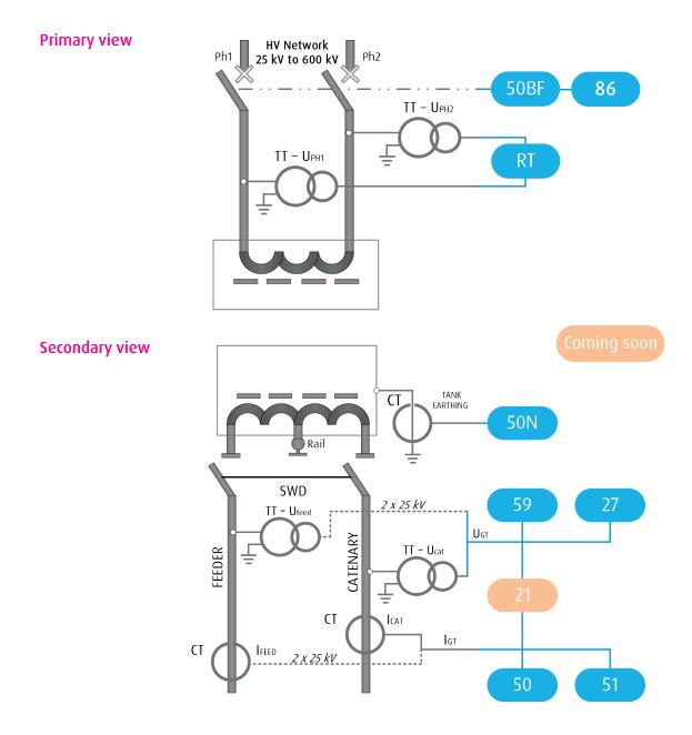
NB: [27] / [50] / [51] / [59] functions can work on both side of the transformer.
