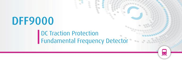
Our DFF9000 monitors the presence of 50/60 Hz fundamental frequency harmonics on DC railway electrical networks. Without this detection, the AC harmonics may disturb the power-line communication for signalisation, implying impact on the railway traffic.
