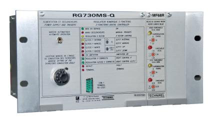
The digital Automatic Voltage Regulator RG730MS-Q is a numerical PID regulator designed to control the excitation of large & medium size synchronous motors.
